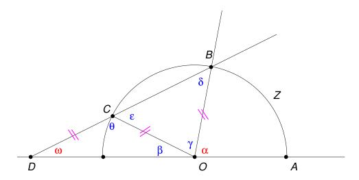
Labelling the angles  $\alpha, \beta, \gamma, \delta, \varepsilon, \theta, \omega$  as shown<sup>2</sup>, it can now be proven that  $\omega = \alpha/3$ . The details are left as an exercise, but the only facts you need are the following:
